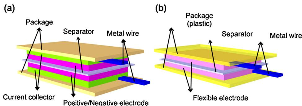
Fig. 4. Schematic illustrations of (a) a traditional supercapacitor and (b) a flexible supercapacitor.
