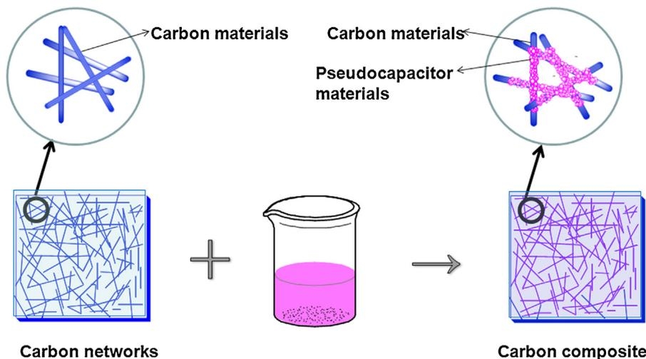
Fig. 3. Fabrication of carbon composites by coating pseudocapacitor materials onto carbon networks through a solution-based method.
