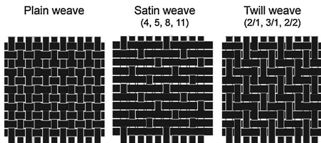
Fig. 2. Three weave styles of carbon fabrics.
